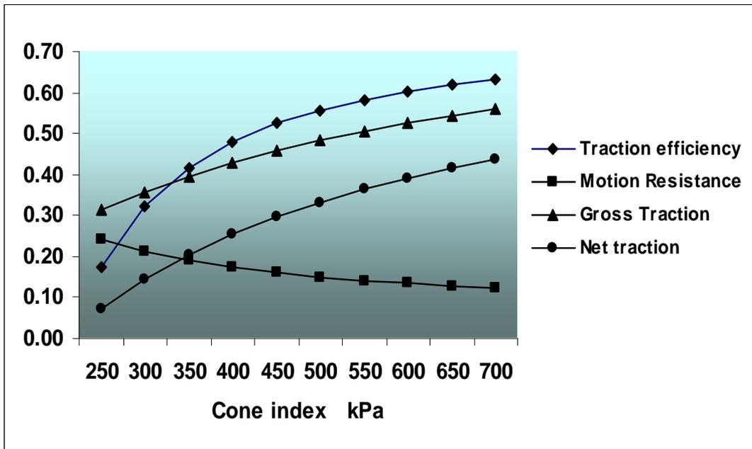
Figure 3 Traction coefficients as a function of cone index.
