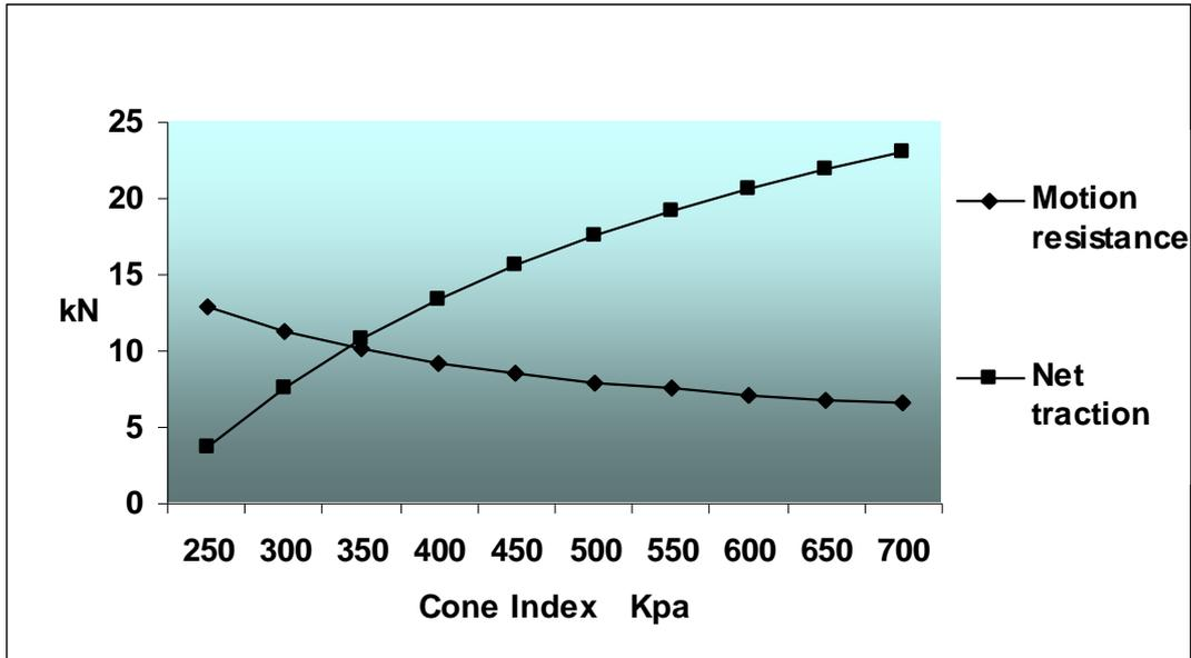
Figure 2 Traction performance as a function of cone index.
