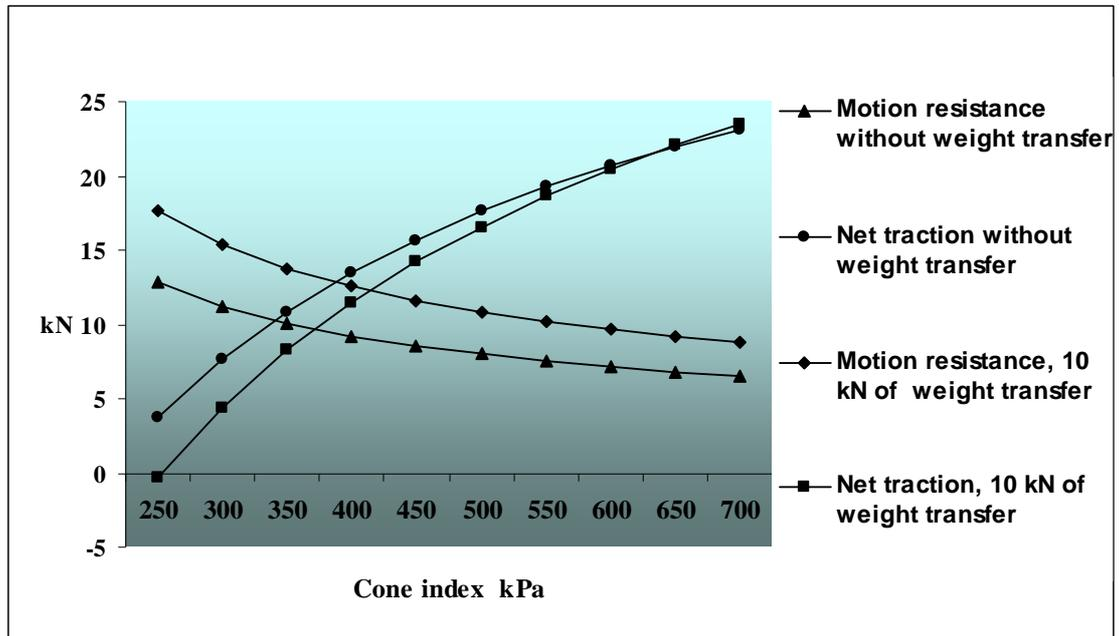
Figure 4 Influence of 10 kN of weight transfer on traction performance.
